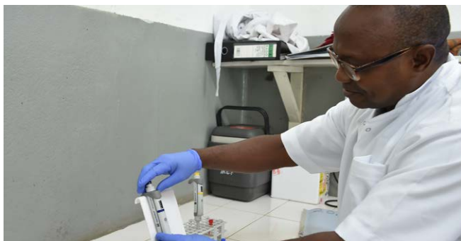
Ministry of Health Laboratory Supervisor, Mamoud Bah, placing a pipette on a 3D printed pipette holder, inside the laboratory of the Magburaka Government Hospital. Photographer: Mohamed Saidu Bah.
