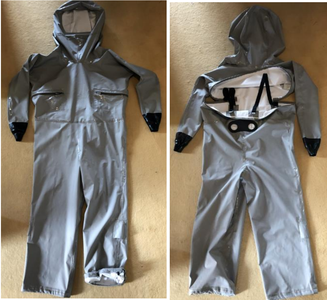
Front and back views showing face shield, watertight zippers, rubber seals and internal suspenders
