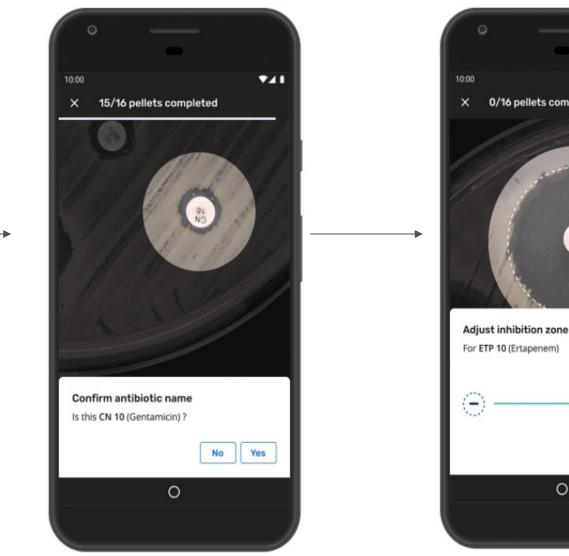
Semi automatic detection of antibiotic discs and measurement of inhibition zone
