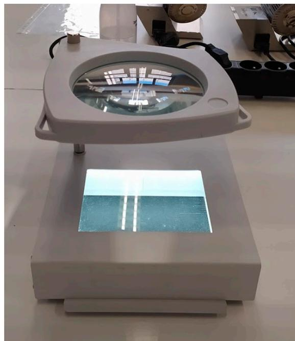
**Figure 2.** Prototype of the microplate viewer by JP Selecta, used for the visual reading. The background at the bottom can be changed to white.
